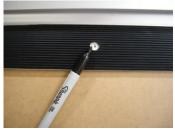
Drill the 2 marked holes with the 6.5mm diameter drill bit provided.
