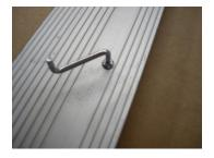
You will need to provide corresponding locating holes at the upper level/step that the ramp will rest on. The locating holes in the upper level/step should be approximately 10mm (3/8") diameter and spaced to match the distance between the locating studs on the deployed ramp. For a step with a square edge/nosing the centre of the locating holes should be 42mm (1 5/8") from the front edge of the upper level/step that the ramp will rest on. Please check as your application may differ.
